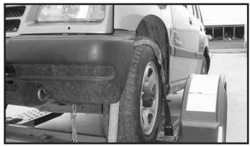
**Step 8**. Be sure tie-down winch is centered with the tire before tightening straps.
